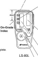
Two on-grade precision options are available, normal precision (±2mm) and high precision (±1mm). By pressing this switch, the precision options are switched alternately. Confirm the precision choice by the indicator. (Normal precision is the default setting each time the sensor is turned on.) Indicator
